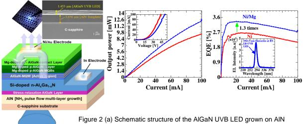
Figure 2 (a) Schematic structure of the AlGaN UVB LED grown on AIN template (b) I-L (in the inset I-V) and (c) I-EQE (in the inset EL Vs
