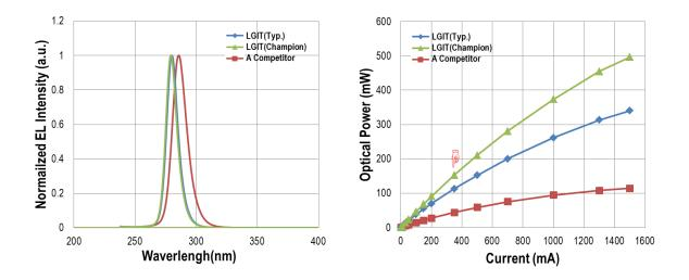
Fig. 1: The EL Spectra of 280nm and Output power vs. Injection current, respectively.
