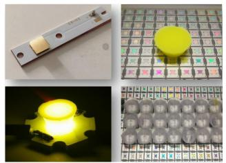
Fig. 1: 3D printed CSP white LED packaging device
