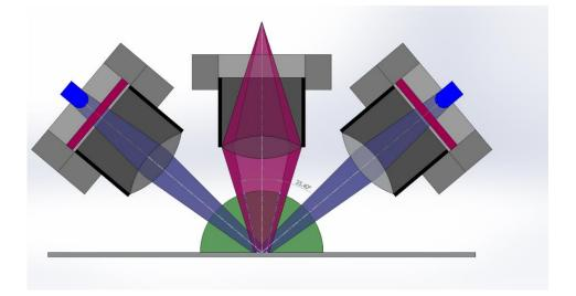
*Fig. 1:* Design of optical path of the experimental model of an autofluorescence based rapid detection of microbial contaminations
