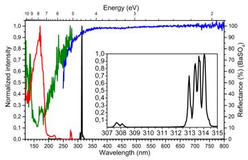
*Fig. 1:* The normalized excitation- $(\lambda_{em} = 314 \text{ nm}, \text{ red line})$ , normalized emission- $(\lambda_{ex} = 160 \text{ nm}, \text{ black line})$ , VUV-reflection- (green line) and reflection-spectra (blue line) of (Lu<sub>2,85</sub>Gd<sub>0,15</sub>)Al<sub>5</sub>O<sub>12</sub> are shown. The inset shows the sample emission from 307 to 315 nm in higher resolution (0.05 nm steps and emission slit).
