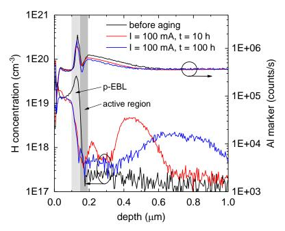
*Fig. 1:* Depth profiles of the hydrogen concentration and the relative aluminum concentration in the heterostructure of a UV-B LED chip before operation and after operation at 20 °C and 100 mA for 10 h and 100 h, respectively.
