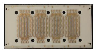
Fig. 2: UVB LED array used for phototherapy
