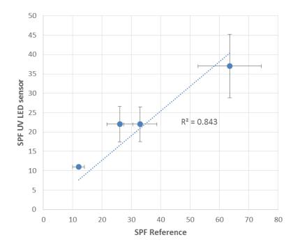
Fig. 1: Comparison of the SPF values of 4 different creams determined by the noninvasive LED reflectance based device and the reference method based on the erythema measurement on the back of volunteers. The error bars correspond to standard error of the mean (SEM, n = 3 to 6). In case of the reference values the maximally allowed SEM according to ISO 2444:2010 is shown, in order to symbolize the uncertainty of the reference values.
