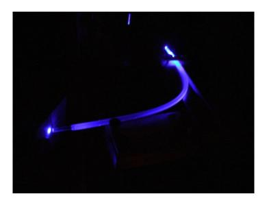
Fig. 1: UV – VIS light propagation in Teflon polymer tubes
