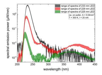
*Fig. 1:* Spectral power density of 233 nm, 229 nm, and 225 nm LEDs measured on-wafer at 20 mA. The parasitic luminescence at ~400 nm and ~275 nm is attributed to deep level transitions ( $V_N^{3+} \rightarrow Mg^0$ ) within the Al<sub>0.2</sub>Ga<sub>0.8</sub>N:Mg layers of the p-superlattice and the last barrier, respectively.
