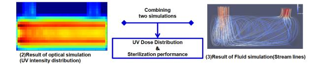
*Fig. 1:* Combining optical and flow simulations to predict disinfection performance in UVC LED-based water disinfection modules.
