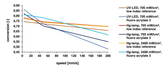
*Figure 1.* Conversion of low index reference material and developed fluoro acrylate 3 in dependence of irradiation speed and light source (UV-LED 390 nm/ Hg-lamp).
