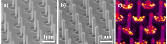
*Fig. 1:* (a) AIN nanorod array after ICP dry etching and KOH based wet etching. (b) AIN nanorod array after AIN MOVPE regrowth. (c) Intensity map extracted from AIGaN/AIN single quantum well core-shell structures over an emission range of 4.9-5.5eV.
