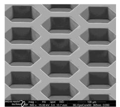
Fig. 1: EpoCore layer, 50 µm thick, exposed with UV-LED @ 365 nm
