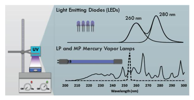
Figure 1. Emission spectra for traditional UV sources compared to UV LEDs. Credit: S.E. Beck, 2017
