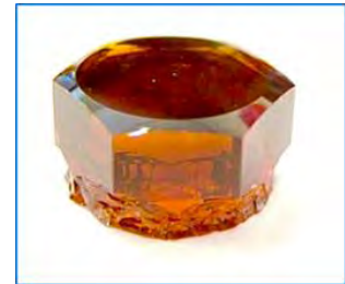
Fig. 1: AlN crystal, 8mm diameter
