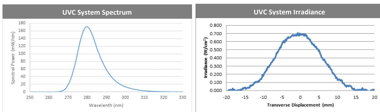
Fig. 1: UVC system with its spectrum (left side) and its irradiance (right side)
