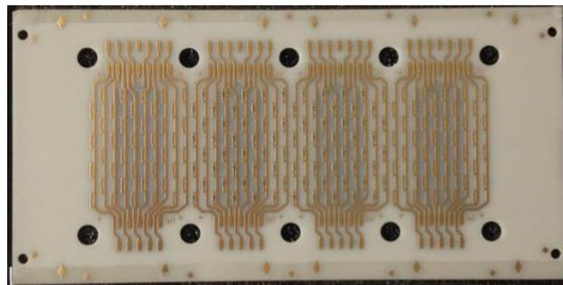
*Fig. 2: UVB LED array used for phototherapy*
