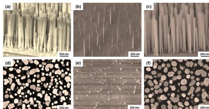
*Fig. 1:* SEM images show that there is inconsiderable reduction of length and diameter of the capped NWs (c,f) w.r.t uncapped and unannealed one (a,d). However, there is significant reduction of length and diameter of the NWs which were annealed without capping (b,e).
