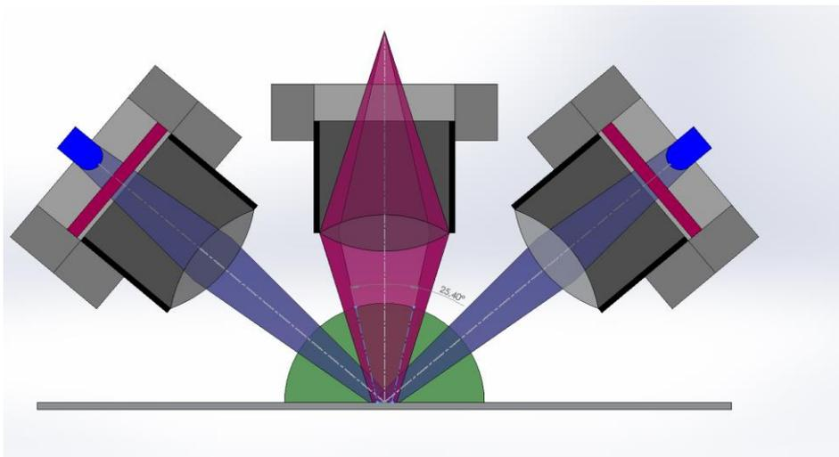
Fig. 1: Design of optical path of the experimental model of an autofluorescence based rapid detection of microbial contaminations
