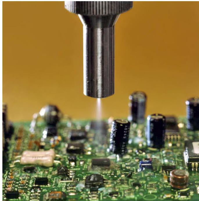
*Fig. 1: Spraying of LED curable 100% solid very low viscosity conformal coating*
