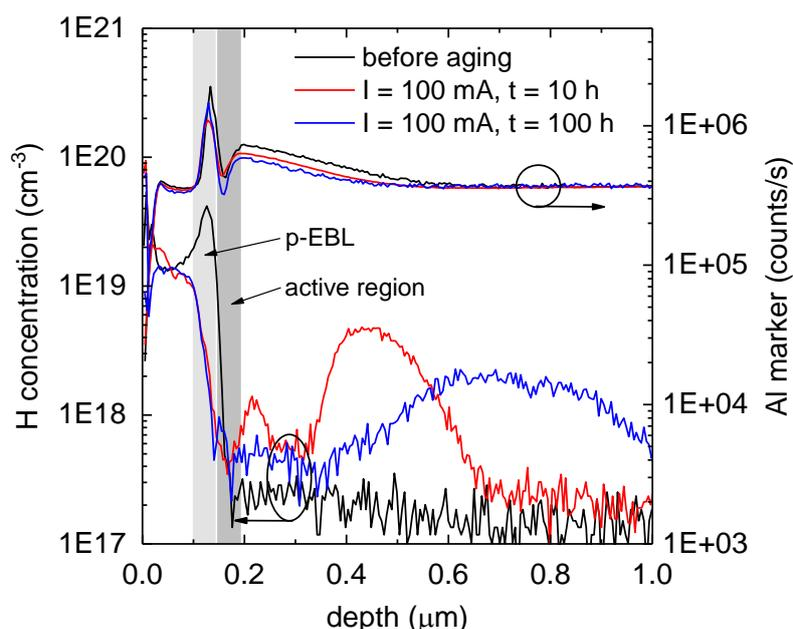
Fig. 1: Depth profiles of the hydrogen concentration and the relative aluminum concentration in the heterostructure of a UV-B LED chip before operation and after operation at 20 °C and 100 mA for 10 h and 100 h, respectively.
