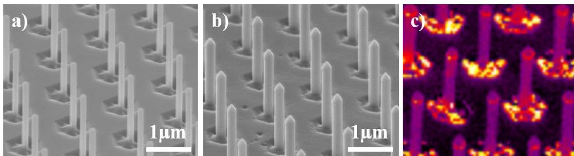
*Fig. 1:* (a) AlN nanorod array after ICP dry etching and KOH based wet etching. (b) AlN nanorod array after AlN MOVPE regrowth. (c) Intensity map extracted from AlGaN/AlN single quantum well core-shell structures over an emission range of 4.9-5.5eV.
