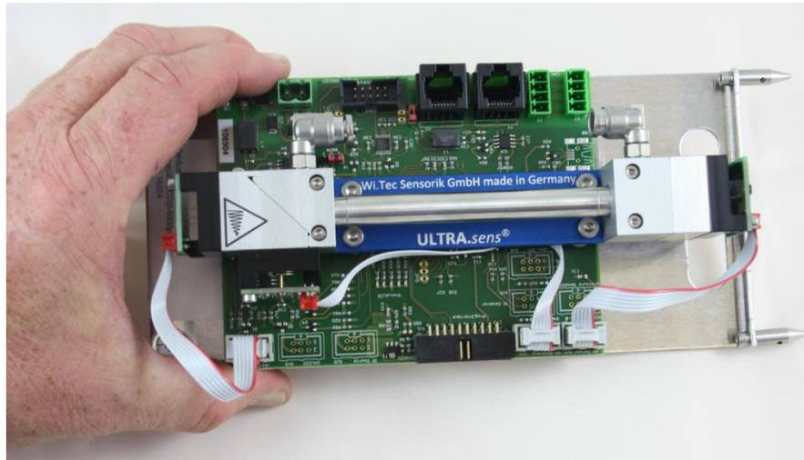
Fig. 1: ULTRA.sens<sup>®</sup> detector for simultaneous analysis of low level SO<sub>2</sub> and NO<sub>2</sub> concentration in flue gas
