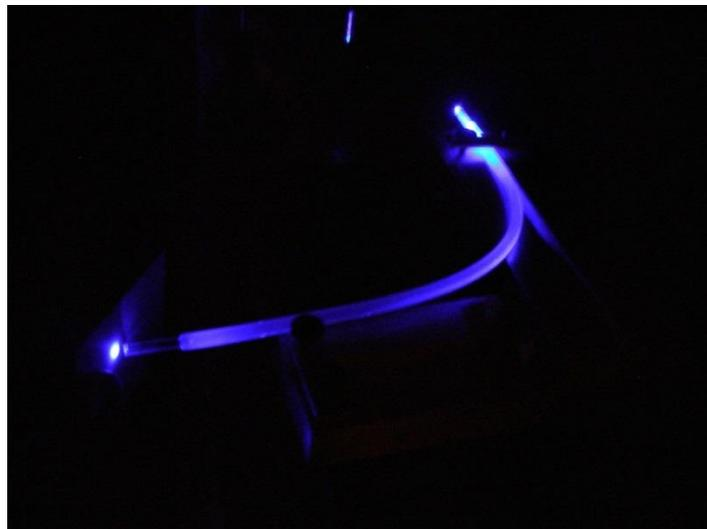
Fig. 1: UV – VIS light propagation in Teflon polymer tubes
