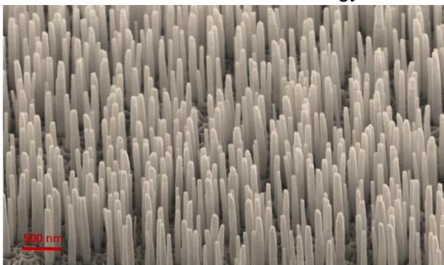
Figure 1. SEM image of AlGa<sub>N</sub> Nanowire.
