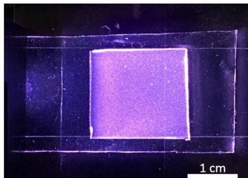
*Fig. 1.* Light sheet with embedded scattering particles coupled to a UV LED (385 nm) in an edge-lit configuration from the left side
