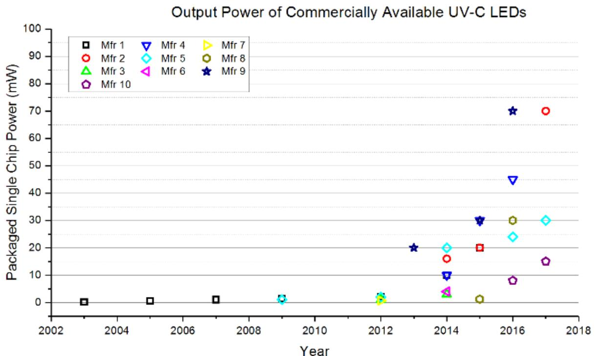
Fig. 1: Output Power of Commercially Available UV-C LEDs
