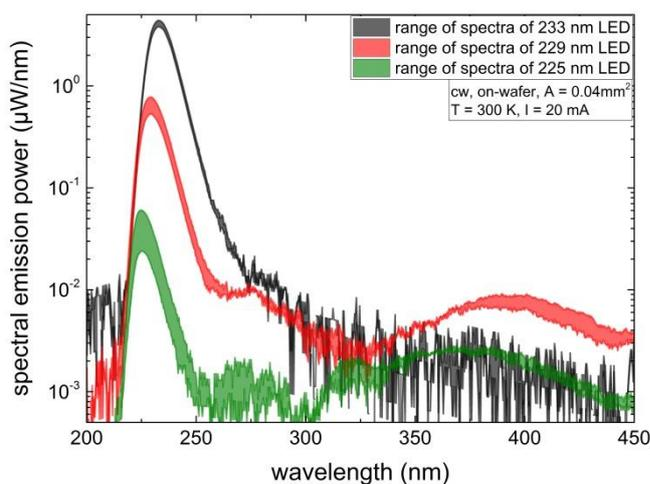
*Fig. 1:* Spectral power density of 233 nm, 229 nm, and 225 nm LEDs measured on-wafer at 20 mA. The parasitic luminescence at  $\sim 400\text{ nm}$  and  $\sim 275\text{ nm}$  is attributed to deep level transitions ( $V_N^{3+} \rightarrow Mg^0$ ) within the Al<sub>0.2</sub>Ga<sub>0.8</sub>N:Mg layers of the p-superlattice and the last barrier, respectively.
