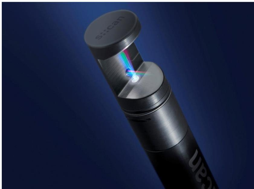
*Fig. 1:* Illustration of the i::scan. Transmitted and scattered light are measured simultaneously using two independent detectors.
