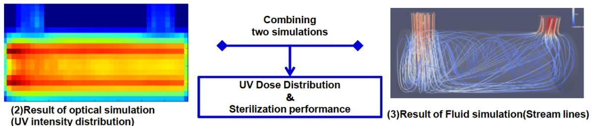
Fig. 1: Combining optical and flow simulations to predict disinfection performance in UVC LED-based water disinfection modules.
