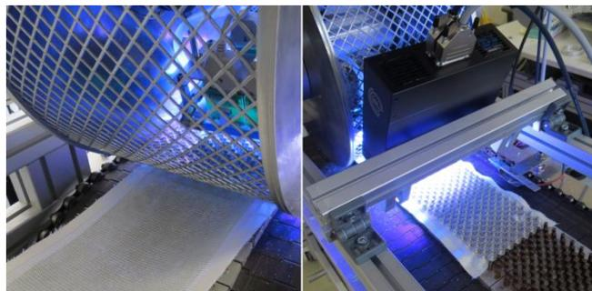
Figure 1: Test plant for nap-core manufacturing
