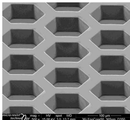
Fig. 1: EpoCore layer, 50 µm thick, exposed with UV-LED @ 365 nm
