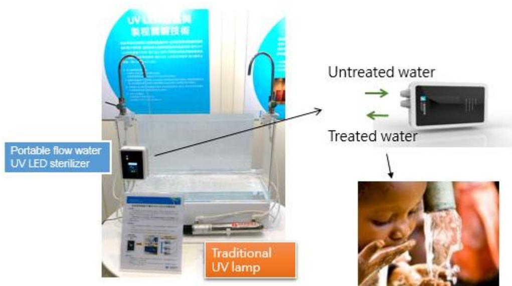
Fig. 1: UVC LED portable flow water sterilizer
