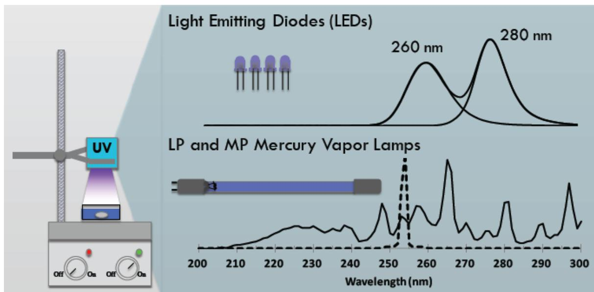
Figure 1. Emission spectra for traditional UV sources compared to UV LEDs. Credit: S.E. Beck, 2017
