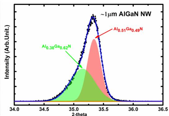
Figure 2. XRD of AlGa<sub>N</sub> Nanowire.
