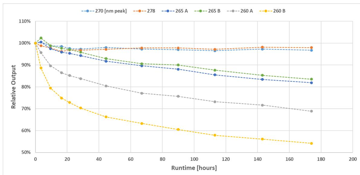
Fig. 1: Loss in UV-output of six different LED-modules due to aging at 22°C.
