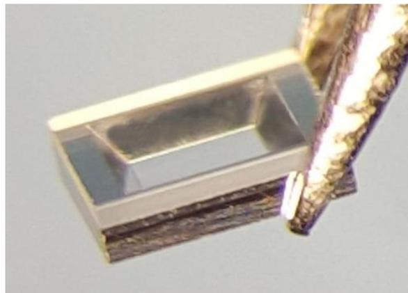
Fig. 1: Macroscopic picture of reflector cap for SMD-packaging
