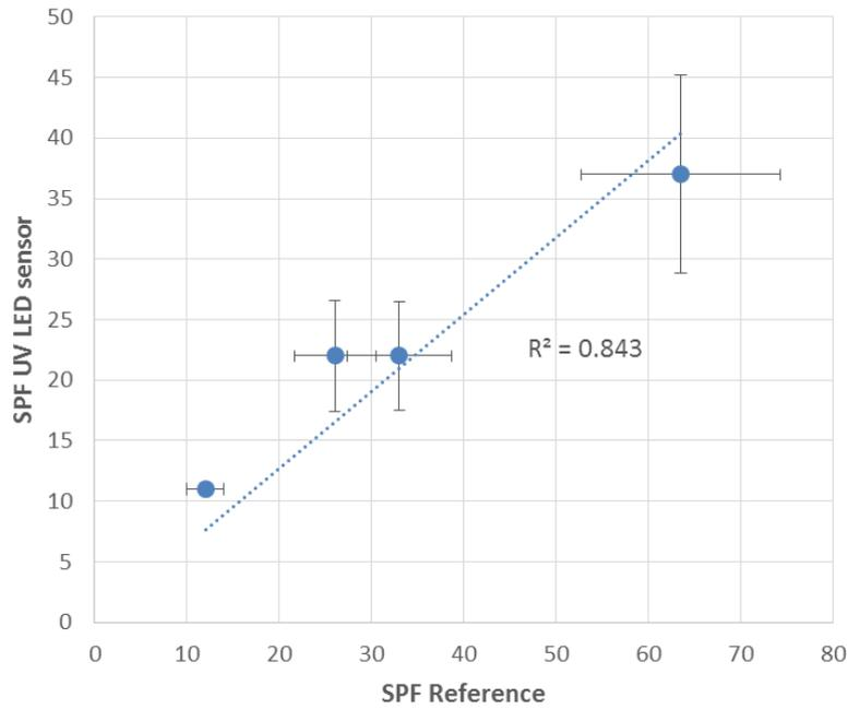
*Fig. 1: Comparison of the SPF values of 4 different creams determined by the non-invasive LED reflectance based device and the reference method based on the erythema measurement on the back of volunteers. The error bars correspond to standard error of the mean (SEM, n = 3 to 6). In case of the reference values the maximally allowed SEM according to ISO 2444:2010 is shown, in order to symbolize the uncertainty of the reference values.*
