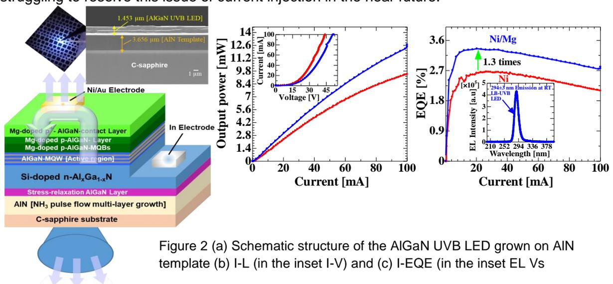
Figure 2 (a) Schematic structure of the AlGaIn UVB LED grown on AlN template (b) I-L (in the inset I-V) and (c) I-EQE (in the inset EL Vs
