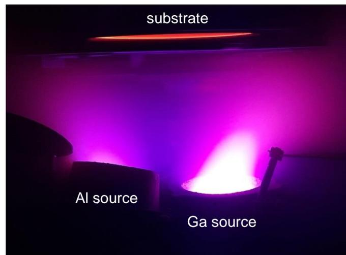
*Fig. 1:* Image of the sputter deposition with the heated substrate at the top. The co sputtering of Al und Ga is done in sputter up geometry. Due to the liquid Ga the right source is horizontal.
