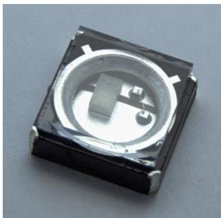
*Fig. 1: UVB LED in an AlN ceramic carrier*
