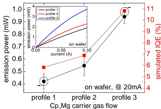
Fig. 1: Measured average emission power as well as simulated internal quantum efficiency (IQE) of 310 nm LEDs with different temporal Cp<sub>2</sub>Mg carrier gas flow profiles (p-doping profiles) in the EBL. Inset: Typical emission power vs. current characteristics of 310 nm LEDs with different temporal Cp<sub>2</sub>Mg carrier gas flow profiles in the EBL.
