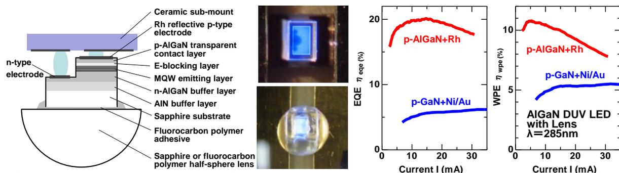
Fig. 1: Structure, photo images, EQE characteristics of AlGaN DUV LED with lens. (The samples were supplied by DOWA Electronics Materials Co. Ltd.)
